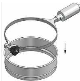
Clamping ring and converter before using the test sieve to be stimulated
